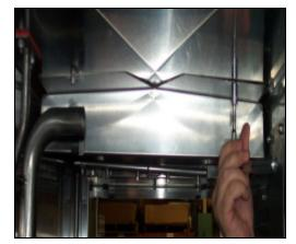
Removing and turning splash shield
